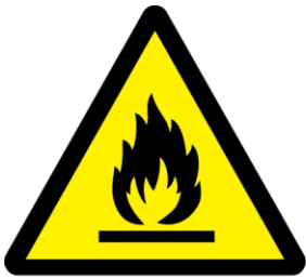
Caution, risk of fire, R290
